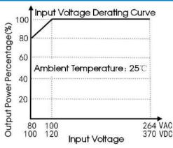
Note: 1) With an AC input between 80-100VAC and a DC input between 100-120VDC, the output power must be derated as per temperature derating curves; 2) This product is suitable for applications using natural air cooling; for applications in closed environment please consult factory or one of our FAE.
